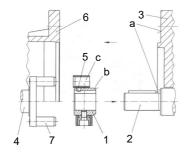
coupling and the coupling shaft (4). Tighten the radial locking screw (5) in the hub. Place the motor on IEC-Adapter (6). Ensure that the socket pins (7) have been correctly inserted into the bore holes (c) of the coupling ring. Fix the motor at the IEC adapter.
